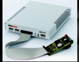
Consists of a "pod" that holds or replaces the processor and a "chassis" that contains specialized debugging hardware, including a trace buffer.
